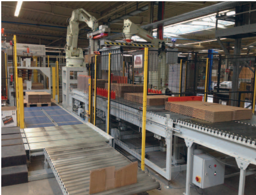
BOX PLANTS IN EUROPE ARE HIGHLY AUTOMATED WITH MATERIAL HANDLING SYSTEMS ON THE FRONT AND BACK END OF EVERY MACHINE CENTER.
