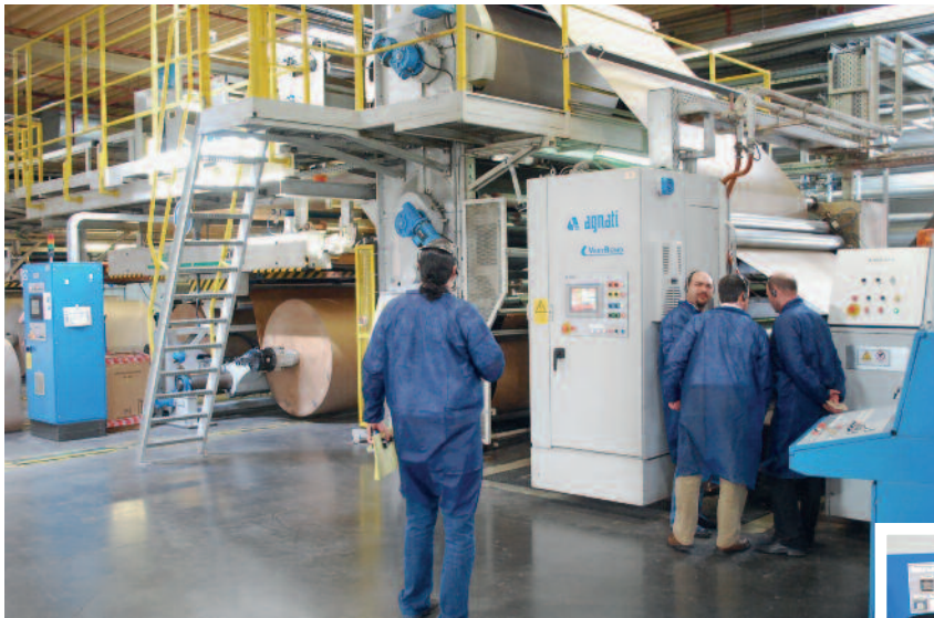
COOLER CORRUGATING TEMPERATURES ARE KEY WHEN RUNNING LIGHTER WEIGHT RECYCLED GRADES. AT BROHL WELLPAPPE THE GROUP WAS GIVEN THERMOMETERS TO CHECK THE TEMPERATURE AT THE SINGLEFACER AND DOUBLEBACKER.
