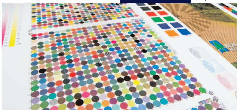
On manual set presses keep copious notes. Record every bit of information it is possible to save. Nip settings, pull roll positions, feed gate positions, vacuum settings, etc. should be recorded for future use.
