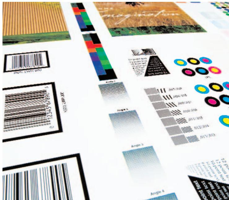
**Test images should be designed to one particular press, and the number of colors in the image should reflect the number of print stations in the press.**
